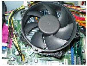
**17.** Disconnect the CPU Cooler power-cable from the MB connector.
